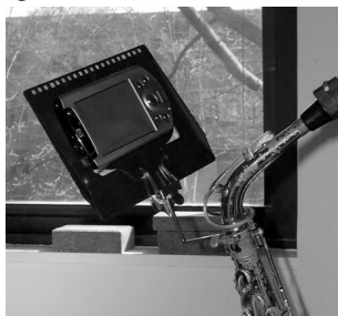
Figure 2. PocketPC PDAs are mounted on each saxophone to display the music notation.
